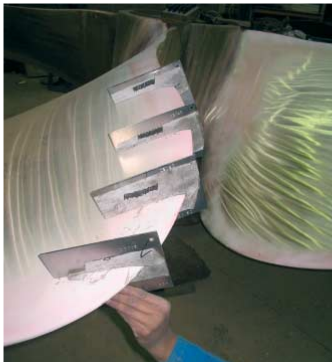
Checking modified trailing edge profile section by means of templates.
