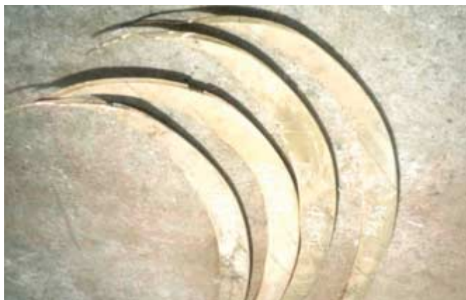
Equal pieces of propeller material are cut off.
