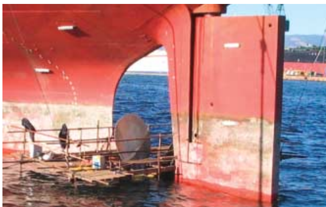
Trailing edge adjustment at pier side.
