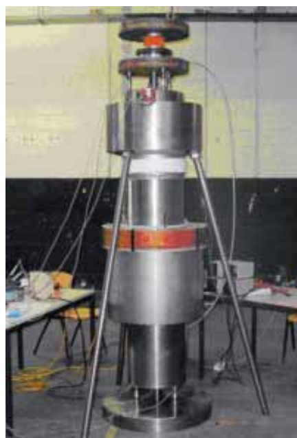
■ Fig. 3 – Thrust sensor on a calibration test bench.
