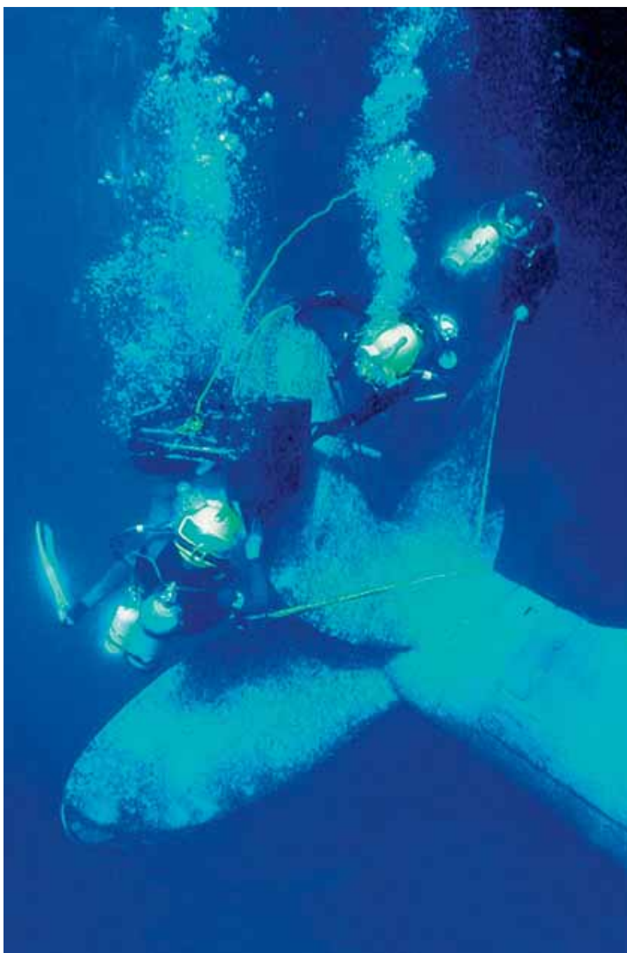
■ Fig. 1 – A Wärtsilä Services propeller polishing team at work.
