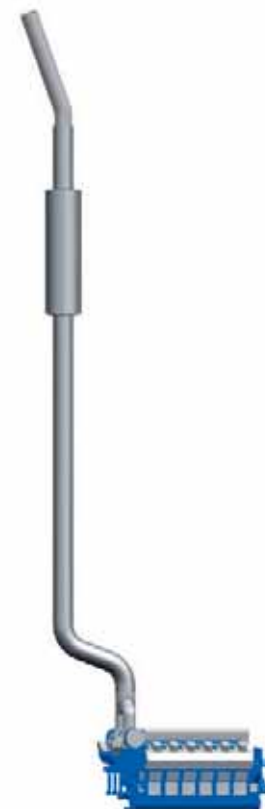
■ Fig. 2 – Conventional silencer system.
