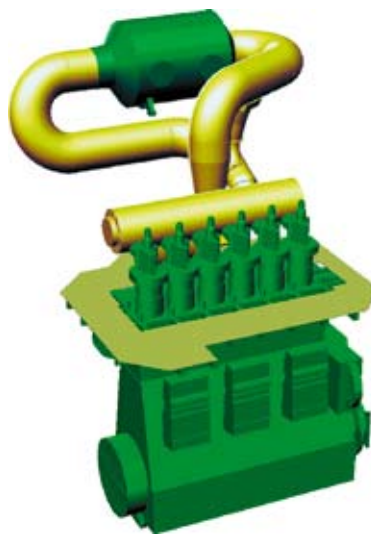
■ Fig. 4 – Arrangement of an SCR plant (cylindrical vessel at the top) between the engine's exhaust gas manifold and turbocharger on a Wärtsilä low-speed engine. This indicates the relative space requirement for the SCR plant.
