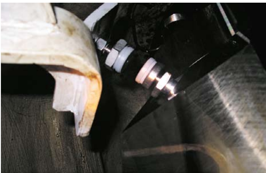
■ Fig. 3 – Big end bearing wireless sensors and their fixture bracket.
