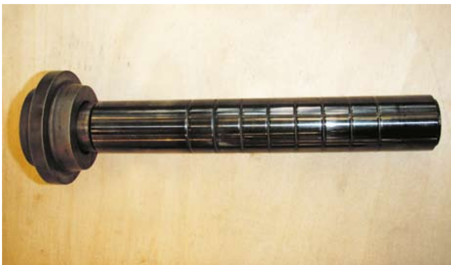
■ Fig. 2 – A pump plunger at the 24,000 hr inspection with no detected cavitations or wear.
