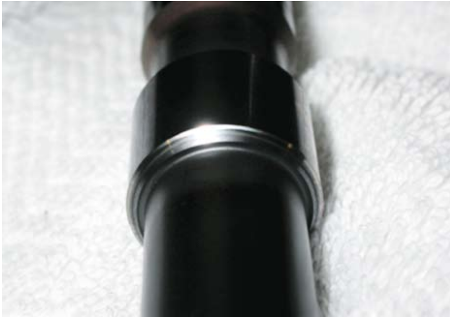
■ Fig. 3 – The latest design version of the shuttle valve is in excellent condition after more than 9220 running hours.
