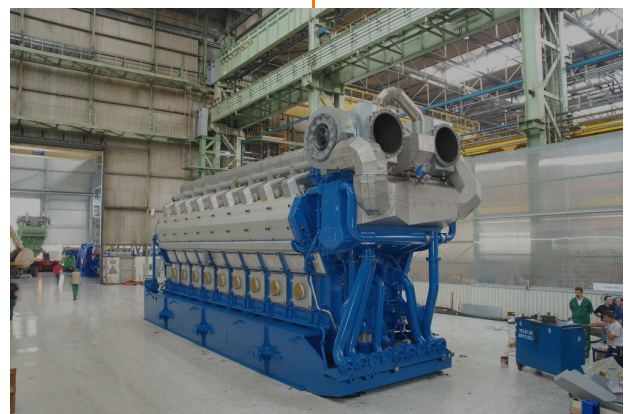
4.5. Wärtsilä 50DF engine successfully demonstrates its capability to operate on ethane gas.
