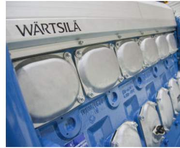
9.10. Wärtsilä 20DF, another ECA compliant dual-fuel engine released to the US market.
