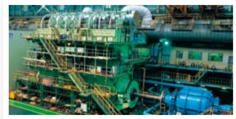
The first engine employing Delta Tuning is this 45,760 kW Sulzer 8RT-flex96C engine seen here in the course of erection at HSD Engine Co Ltd., Korea.
