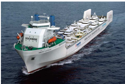
“Dockwise Yacht Carrier.” 2 x Wärtsilä 8L38B 2 x Wärtsilä 4L20 1 x Wärtsilä 9L20 2 x LIPS CS3500 Steerable Thrusters 1 x LIPS CT225 Tunnel Thruster
