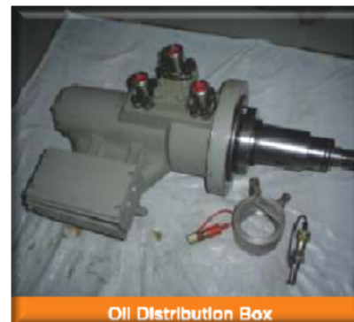
Oil Distribution Box
